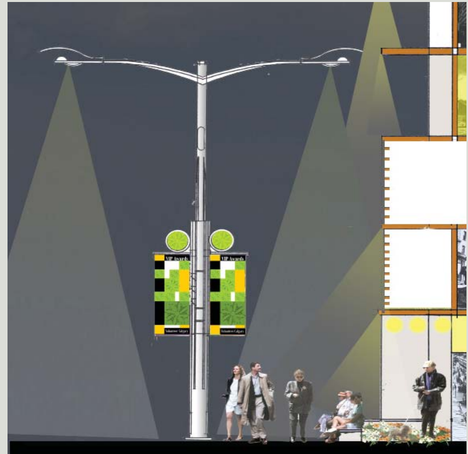
Image 36: An illustration showing design to constrain light to the features being lit..
